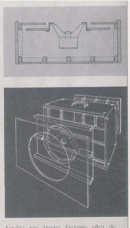
Fender's new Speaker Enclosure offers the finest in amplified sound reproduction. The Speaker Projector Ring<sup>9</sup> employed eliminates cancellation of front and rear radiation, thus permitting greater speaker efficiency and optimum performance of the enclosure.
